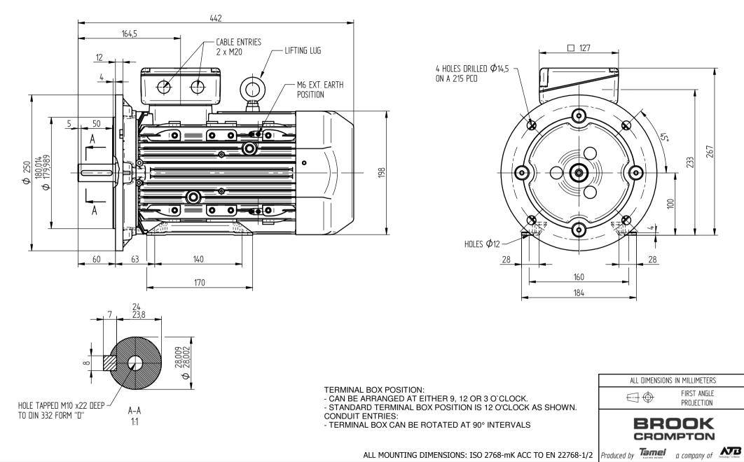
SHEET SIZE A3 OUTLINE DIMENSIONS DRAWING TOTALLY ENCLOSED FAN-COOLED WP-DA100LF FRAME D FLANGE AND FOOT MOUNTED MOTOR.
