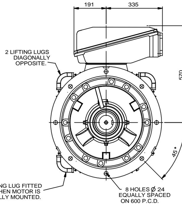
THIS LIFTING LUG FITTED ONLY WHEN MOTOR IS VERTICALLY MOUNTED.
