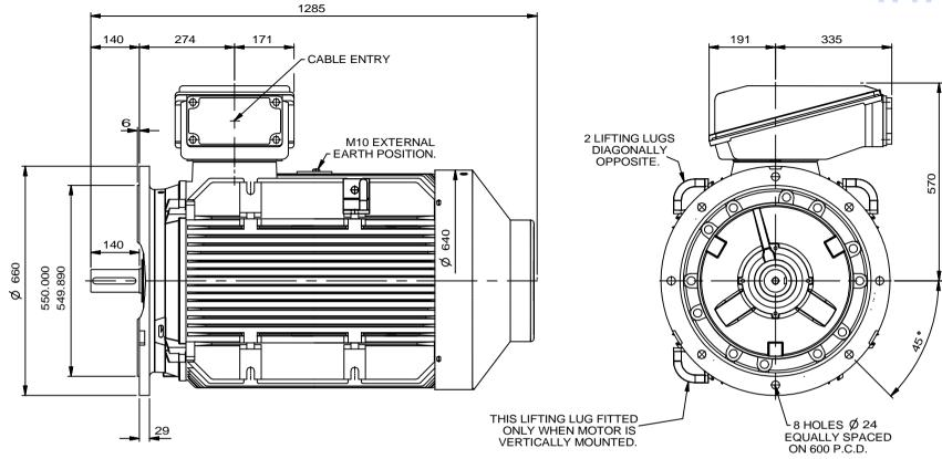
NOTE! CABLE ENTRY CAN BE SUPPLIED IN ANY ONE OF FOUR POSITIONS AT 90° INTERVALS.
