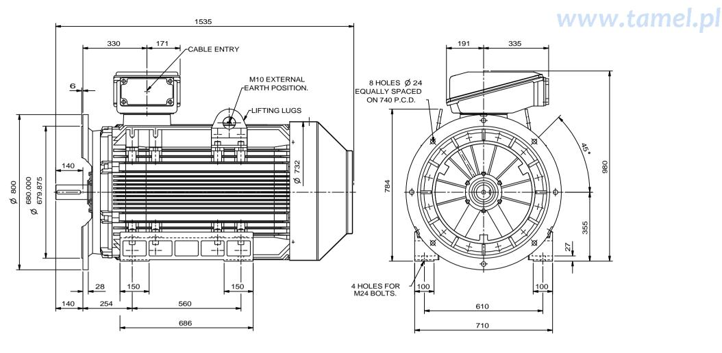
NOTE! TERMINAL BOX CAN BE SIDE MOUNTED (LEFT OR RIGHT) BY REFITTING FEET 90° IN APPRÓPRIATE DIRECTION. CABLE ENTRY CAN BE SUPPLIED IN ANY ONE OF FOUR POSITIONS AT 90° INTERVALS.
