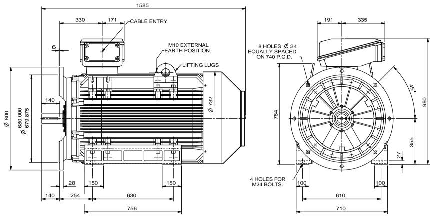
NOTE! TERMINAL BOX CAN BE SIDE MOUNTED (LEFT OR RIGHT) BY REFITTING FEET 90° IN APPROPRIATE DIRECTION. CABLE ENTRY CAN BE SUPPLIED IN ANY ONE OF FOUR POSITIONS AT 90° INTERVALS.
