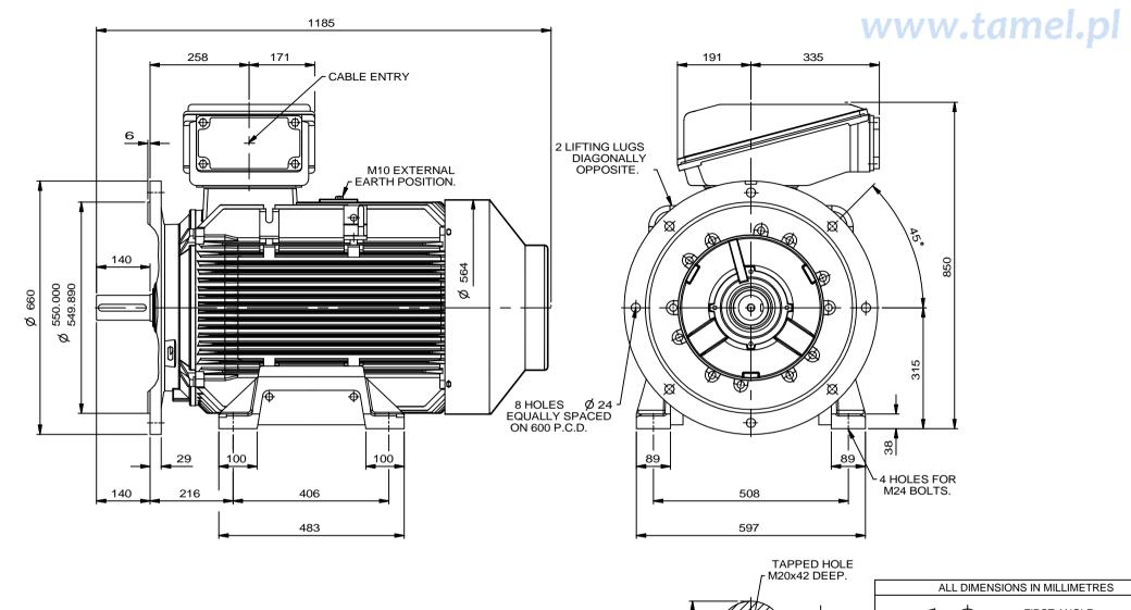
NOTE:-TERMINAL BOX CAN BE MOUNTED (LEFT OR RIGHT) BY REFITTING FEET AND LIFTING LUGS 90° IN APPROPRIATE DIRECTIONS. CABLE ENTRY CAN BE SUPPLIED IN ANY ONE OF FOUR POSITIONS AT 90° INTERVALS.
