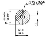
SECTION THROUGH SHAFT EXTENSION (SCALE 1:3.)
