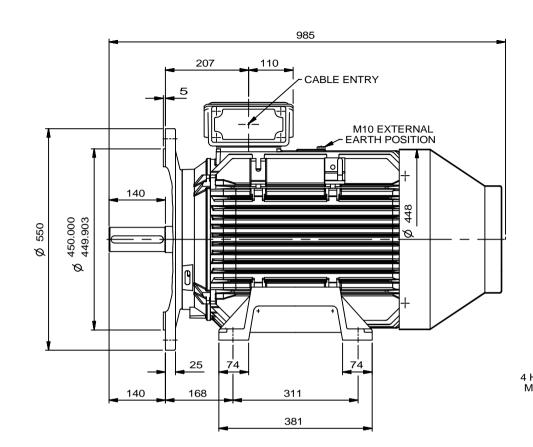
8 HOLES Ø 19 EQUALLY SPACED ON 500 P.C.D. 1 127 250 79 4 HOLES FOR M20 BOLTS. 406 483
