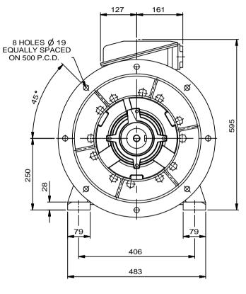
NOTE:-TERMINAL BOX CAN BE MOUNTED (LEFT OR RIGHT) BY REFITTING FEET AND LIFTING LUGS 90 ° IN APPROPRIATE DIRECTIONS. CABLE ENTRY CAN BE SUPPLIED IN ANY ONE OF FOUR POSITIONS AT 90 ° INTERVALS.
