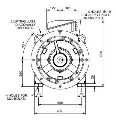
NOTE:-TERMINAL BOX CAN BE MOUNTED (RIGHT OR LEFT) BY REFITTING FEET AND LIFTING LUGS 90 IN APPROPRIATE DIRECTIONS. CABLE ENTRY CAN BE SUPPLIED IN ANY ONE OF FOUR INTERVALS. POSITIONS AT 90
